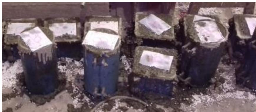
Fig. 4: Casting the Standard Cubes and Cylinders
