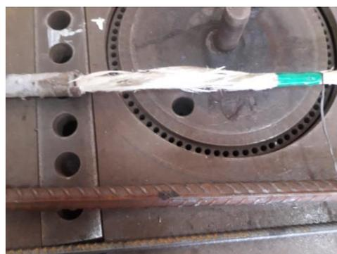
**Fig. 2: GFRP bars during the tensile test.**
