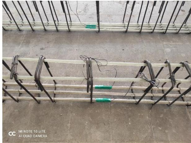
**Fig. 5: the RFT details of tested beams**
