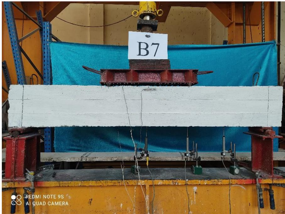
Fig. 7: the test setup of the tested beams
